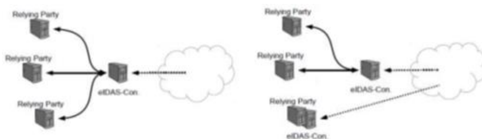
Figure 4: Centralized and decentralized approach[28]
